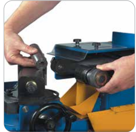
Patented quick-change roller system
