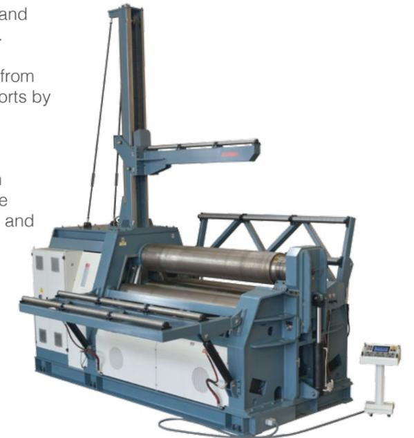
Especially the during bendings of the large diameter and thin material ellipse, parallel corners and polycentric shaped may effect the precisions and can cause deformation of the material, when there is not enough support
