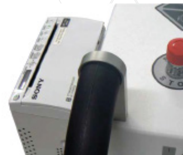
Onboard thermal printer for immediate hardcopy image output*
