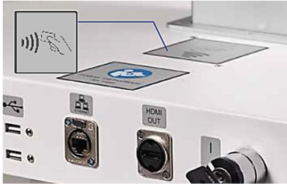
NFC technology, for smart card login
