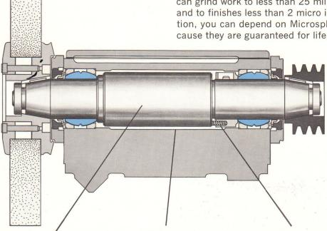
Increased diameter of the spindle between the bearings greatly increases spindle rigidity over conventional single diameter spindles.
