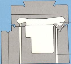
These pockets accumulate the excess of lubricating oil pumped to the ways. Since the pockets are open to atmosphere there is no danger of floating the carriage from excessive pressure.
