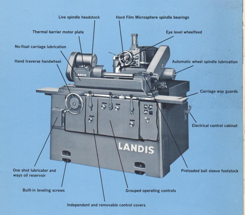
Type 1R grinder with hydraulic traverse and hydraulic infeed
