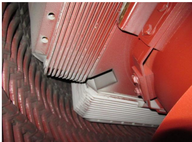
Exciter end rotor and end windings.
