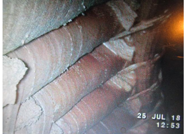
End windings contamination
