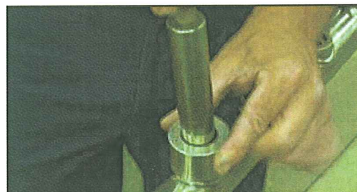
Fig. 4, drive ring in place
