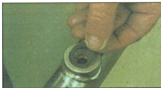
Fig. 1, place the gasket
