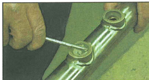
Fig. 5, set the retaining ring
