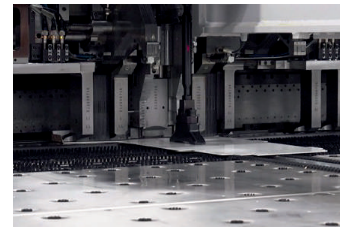
Our Synthesis steel frame panels are made to exact specification on a state-of-the-art bending machine.
