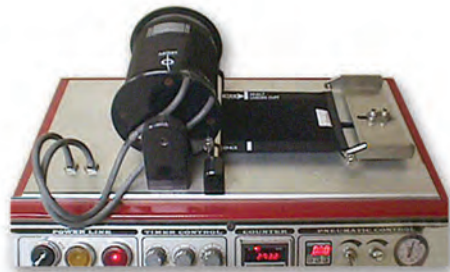
Cuff hook and loop adhesive test
