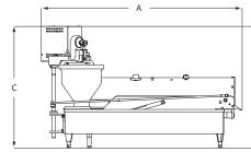
Drawing shows Donut Robot cake donut depositor. Note: Mark VI normally uses Type F depositor.
