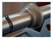
Films with either 57mm or 75mm cores may be used for flexibility of supply.
