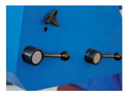
Nip and pull roller pressures are adjusted independently for best results.
