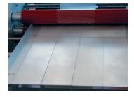
A fully adjustable, positive side lay is provided to aid consistent feeding by hand. The feed table can be easily removed to allow the coupling of an automatic sheet feeder.
