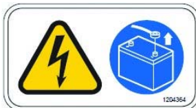
WARNING LABEL - Electrical hazard. Disconnect battery cables before servicing machine.
