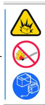
WARNING LABEL - Batteries emit hydrogen gas. Explosion or fire can result. Keep sparks and open flame away when charging. Located on bottom side of recovery tank.
