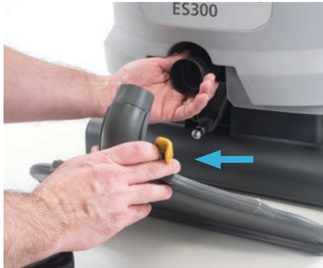
4. Squeeze the lever on Vacuum Shoe to remove the shoe. Rinse the shoe and remove any debris inside the shoe.
