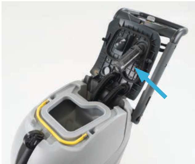
3. Remove and rinse the Recovery Dome Lid. Make sure the Vacuum Mode Selector Knob is turning freely. Rinse the Float Ball & Cage.
