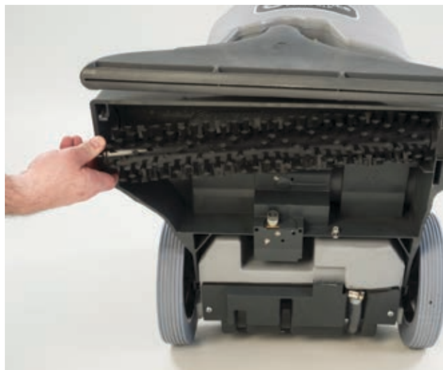
5. Remove the brush by pulling on the left side. Clean the brush of any hair or debris. Inspect the brush for wear and check the brush bearings for hair. Reinstall.
