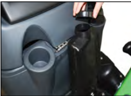
SEPARATE DETERGENT DOSING SYSTEM
