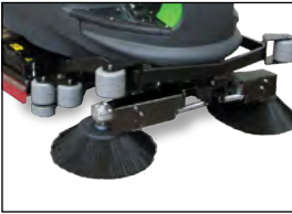
PRE-SWEEP SYSTEM ON CYLINDRICAL MODEL
