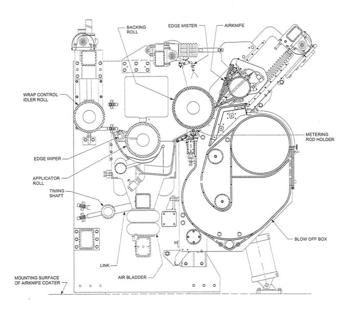
Figure 2-1 Section at Center of Machine
