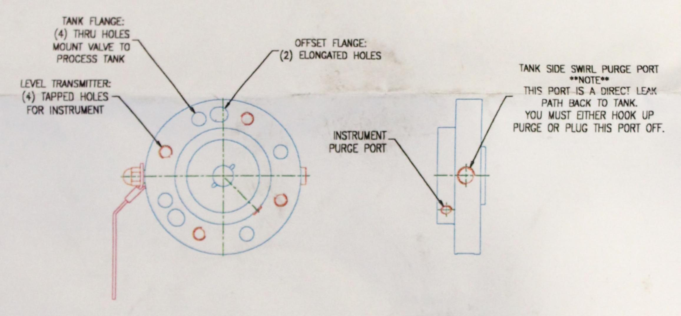
The Indu Tech Isolation Valve has two purge ports:
