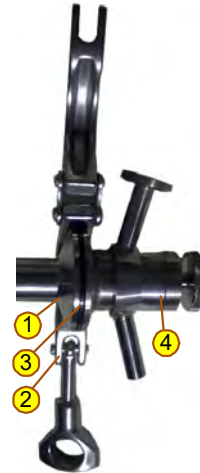
Figure 5-3: The clamp is placed around the aseptic sampling valve /gasket /welding ferrule or threaded male adapter
