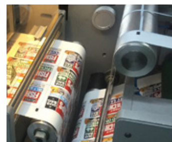
Matrix stripping at a breeze. Two roller design - first a strip roller with anti-stick coating and then a waste rewind. Both with stepless tension.
