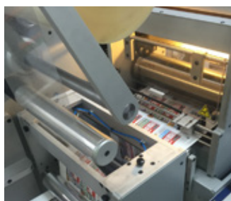
Unwind for self-adhesive unsupported laminates. Fast and trouble free protection of digital print. Optional support paper rewind.
