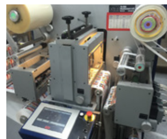
The short distance from unwind to rewind ensures minimum waste of material. The machine is easy to web up due to canterlevered design.
