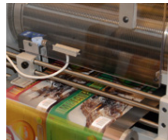
High precision servo controlled semi-rotary die cutter. Perfect re-register to digitally printed webs. Support for marks on transparent web.
