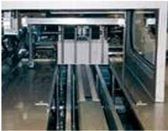
Separating and collection area Separating and collection area with servo operated separation
