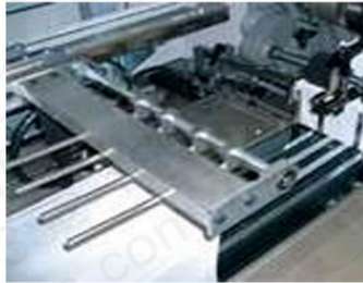
Separation The programmed quantity of envelopes is automatically separated and moved forward as a bundle
