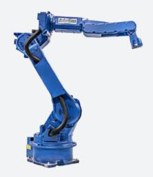
The Motoman EA1900N is a high-performance welding robot that features an internal cable design that was patented to eliminate cable flip. The standard EA1900N NX100 is floor mounted.
