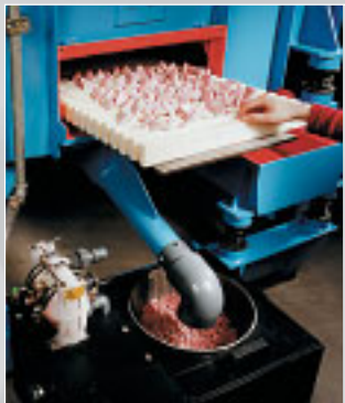
Abrasive media fines separation with collecting zone
