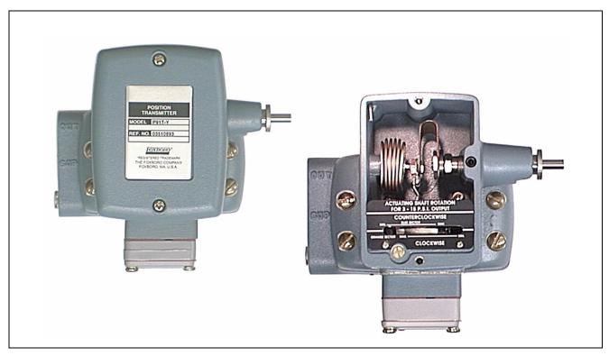
The P91T Pneumatic Position Transmitter measures changes in angular position of its operating lever. It transmits a standard 20 to 100 kPa or 3 to 15 psi pneumatic output signal proportional to either the clockwise or counterclockwise rotation of the lever.
