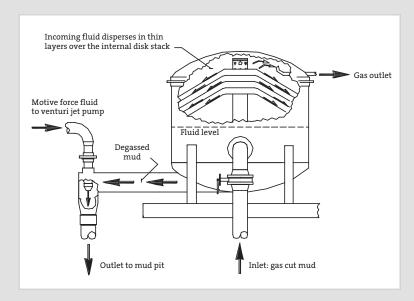
ensure that the disk stack is never submerged. As fluid level rises and lifts the float, air enters the vessel through the three-way valve to decrease the vacuum inside the vessel. With less vacuum inside the vessel, the rate at which fluid is drawn into the tank slows and the rate at which fluid exits the vessel increases. The fluid level inside the vessel drops rapidly until the
