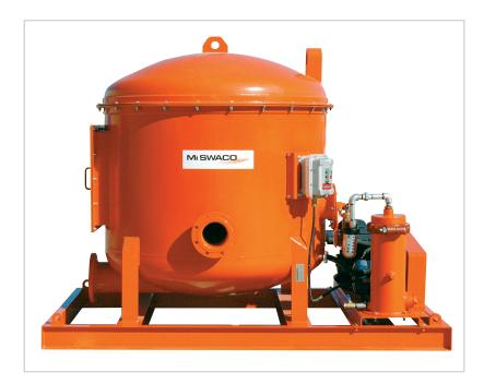
downstream of the sand trap and upstream of any centrifugal pumps. Vacuum degassers work by removing entrained gases from the drilling fluid by exposing the fluid to pressures well below ambient atmospheric pressure.
