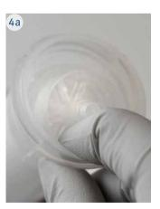
5. Insert the cap with Samplet<sup>®</sup> into the cartridge top and tighten firmly. Ensure the cap is even and fully tightened down, there should be no more than a 1 mm gap between the cap and the mounting fin as shown.
