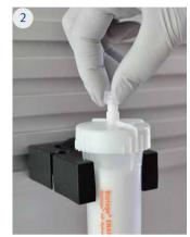
Remove the bottom Luer 3. plug cap.
