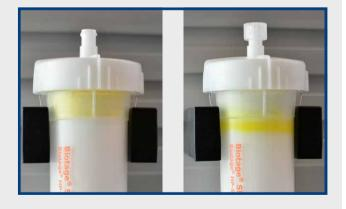
Figure 2. Biotage<sup>®</sup> SNAP Ultra cartridge loaded with a sample pre-adsorbed on silica gel (left) and Biotage HM-N (right). The pre-adsorption on the HM-N renders much tighter bands.
