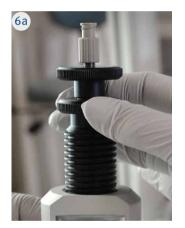
7. Turn the upper nut on the plunger clockwise to lock the o-ring. Finger-tighten.
