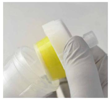
Figure 4. Samplets are placed inside of Biotage<sup>®</sup> SNAP cartridges which maximizes the amount of media available for purification and eliminates and precipitation risk.
