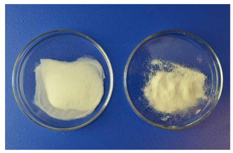
Figure 1. Left: Pre-adsorption on silica gel (3 g, part number K0-1107-05000). Right: Preadsorption on Biotage HM-N diatomaceous earth (3 g, part number 9800-1000).
