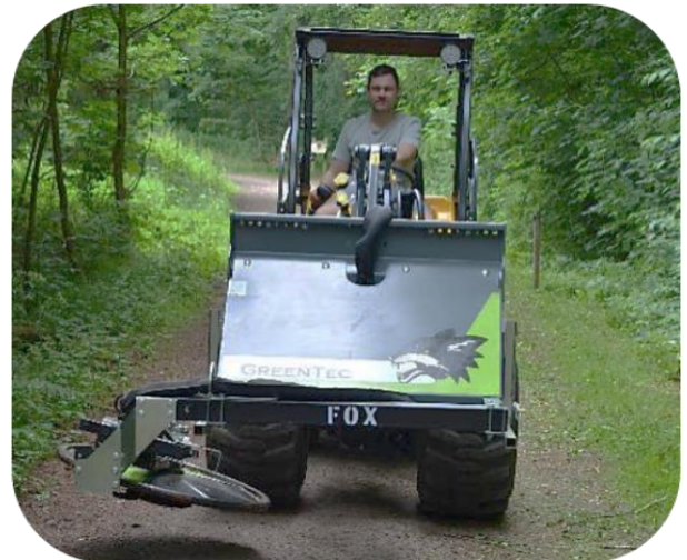
FOX Multi Carrier mounted with RI-80 Barrier Mower in transport position. The Barrier Mower is facing inwards towards the vehicle, for maximum traffic safety.
