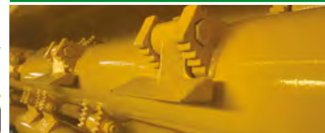
Position of the self-cleaning rear roller for discharging the mulched product behind the roller for higher output
