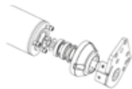
REAR ROLLER PROF Ø 140 mm with 4 bearings with tapered rollers, mud scraper and interchangeable central part.
