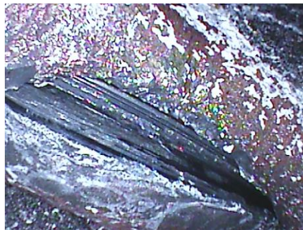
Idle end rotor taper at the tip is grooved.
