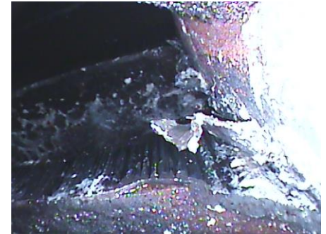
Idle end cone cladding peeled, rotor taper grooved at the tip.
