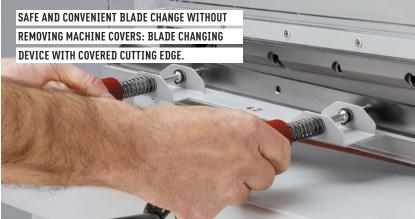
Light beam safety curtain on front table | transparent safety cover on rear table I main switch and safety lock with key I electronically controlled two-hand operation | 24 volt controls (low voltage) | patented IDEAL safety drive I automatic blade and clamp return from every position I disc brake for instant blade stop I easy and safe blade and cutting stick change without removing covers I blade changing device with covered cutting edge I blade depth adjustment from outside of the machine
