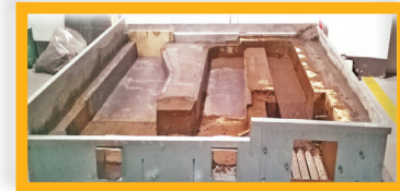
Oven base with hearth and duct system. These components serve as an additional isolator and heat accumulator providing proper distribution.
