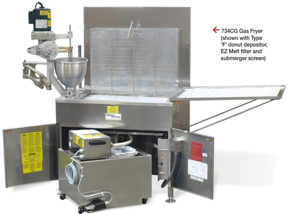
← 734CG Gas Fryer (shown with Type 'F' donut depositor, EZ Melt filter and submerger screen)
