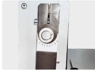
Punch 500 ES and Punch 500 HD models come equipped with eccentric shafts.
