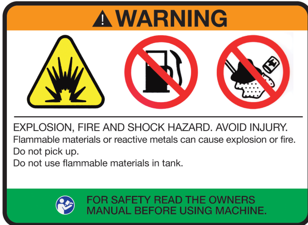
Figure 1: Explosion, fire, and shock hazard label, located in front of the operator seat
