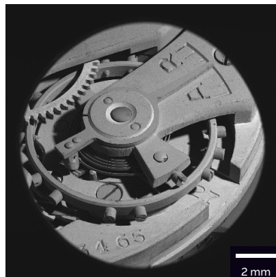
▲ (Left) Image in Overview Mode with field of view of 13 mm and depth of focus over 40 mm. (Right) The WideField Mode offers an extra-large field of view up to 50 mm for live navigation on the sample
