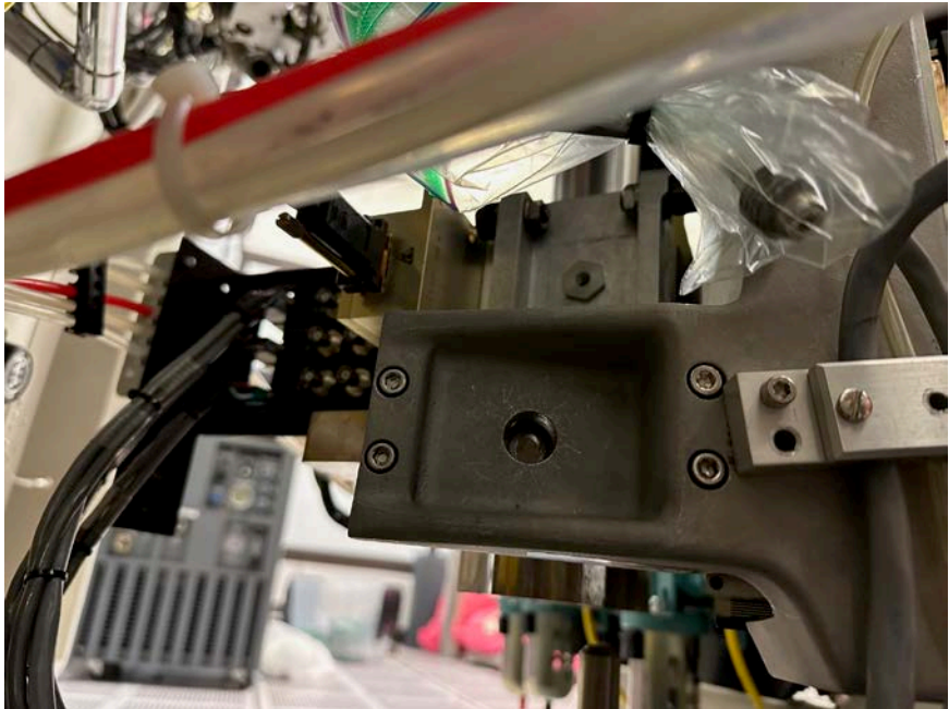
End station air bearing raised and secured for transit (2)
