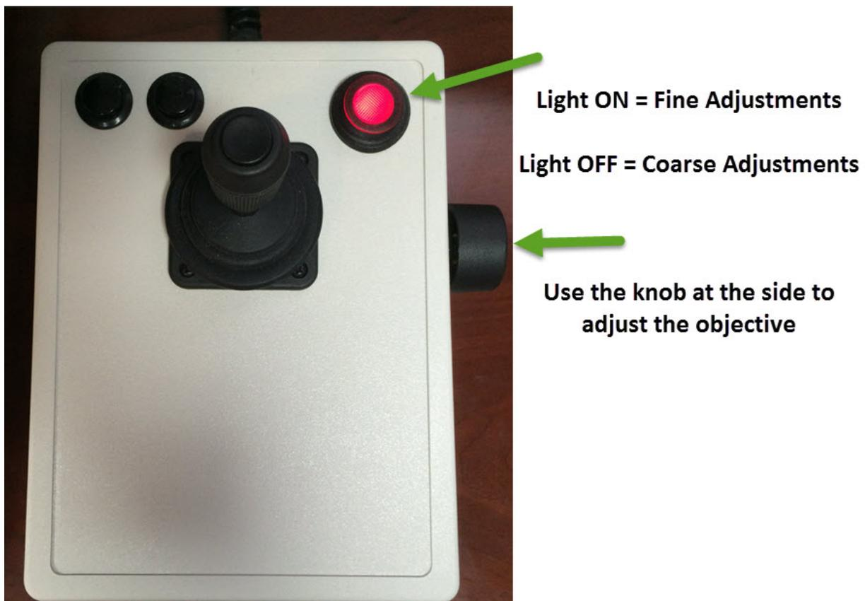
Fig. 2.1: Joystick focus control
