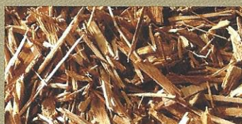
Biofuel from scrap board processed with a 4-inch grate.
