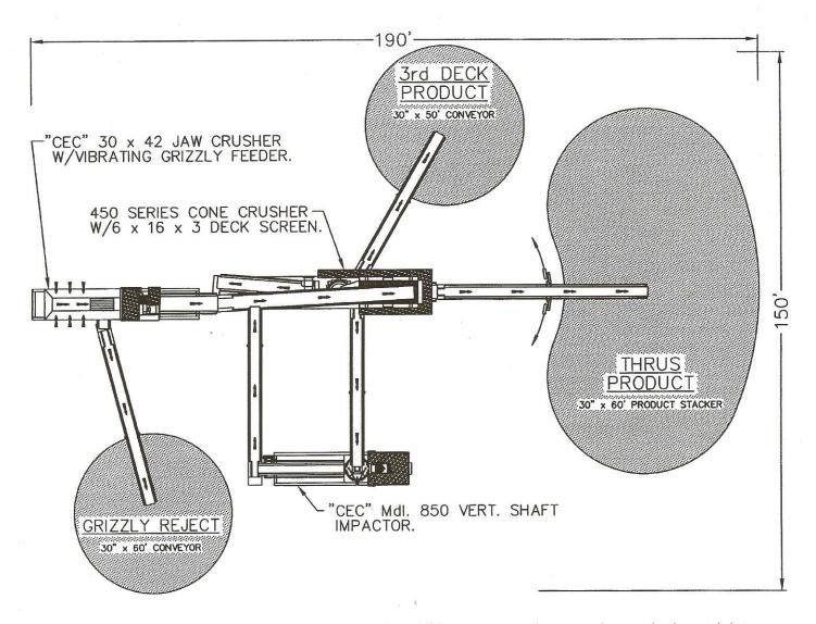
CEC can provide you with a complete plant layout. In addition, we can take your pit sample, insert it into our computer program and provide you with a reasonable estimate of your plant production, product by product, including final gradation.
