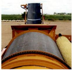
The 510 Cougar has tensioned screen panels which provides a quick clean installation. Maximizing open screening area. The screen panels on the Wildcat Cougar can be changed quicker than any other trommel screen on the market.
