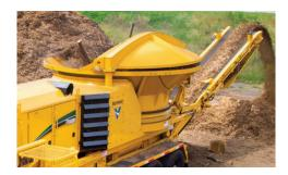
JOBSITE SAFETY. The patented Thrown Object Restraint System (TORS) reduces the amount and distance of thrown objects, and has a smooth underside for better material flow.
