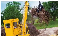
JOB EFFICIENCY. An optional loader cab with grapple increases efficiency and can lift up to 3500 lb (1587.6 kg) at full reach.
