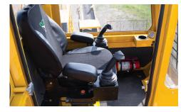
CONTROL IN YOUR HANDS. The loader's electric-over-hydraulic controls provide the flexibility for an operator to use their preferred control configuration (Vermeer, SAE or ISO), as well as three operating modes with varying joystick sensitivity to meet the operator's needs.
