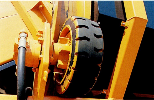
Solid rubber tire drive for less maintenance.
