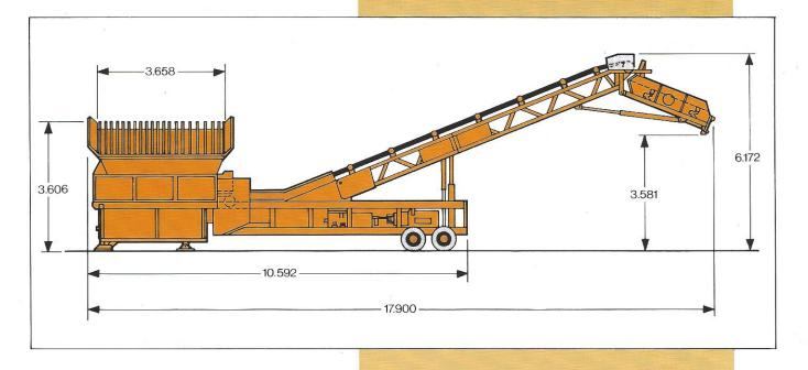
**FEED HOPPER** Capacity 7.5m<sup>3</sup> incorporating heavy duty hopper feeding onto a 1050mm (42") wide belt. Belt speed is adjustable through with variable control speed valve.
