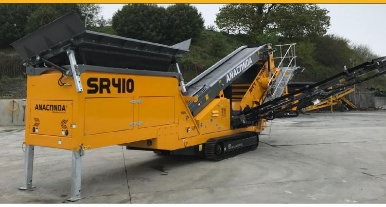
The Anaconda SR Range of Mobile Tracked Finishing Screens have been developed specifically to suit applications where seperating fines is of the upmost importance.
