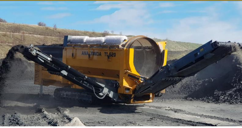
The Anaconda TD Range of Mobile Tracked Trommel Screens are Heavy Duty Cylindrical Screens that has been designed specifically for exceptional results in testing scenario's.
