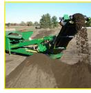
Radial Conveyor Patented radial conveyor with 180° swing and variable discharge height for maximum stockpiling flexibility.
