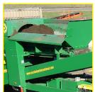
Feed Hopper 2.9m (9' - 6") low load height, large hopper capacity of 3.4m<sup>3</sup> (4.5 yd<sup>3</sup>).
