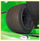
Drum Drive Solid vulcanized, independently powered drive wheels for maximum torque, traction and life.
