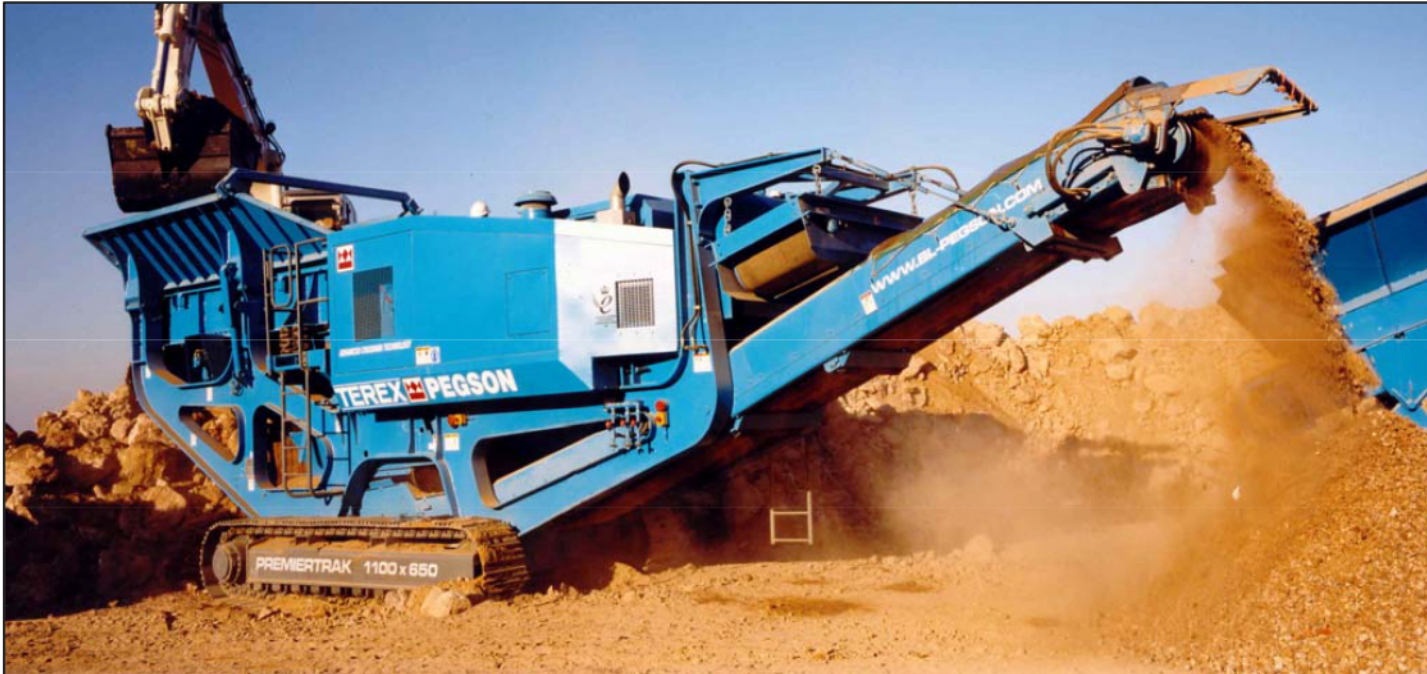
Above image features an 1100 x 650 Premiertrak fitted with the optional side conveyor and overband magnetic separator.
