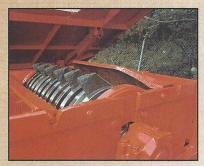
Hydraulic tub tilt feature allows convenient service of the hammermill and screen area.
