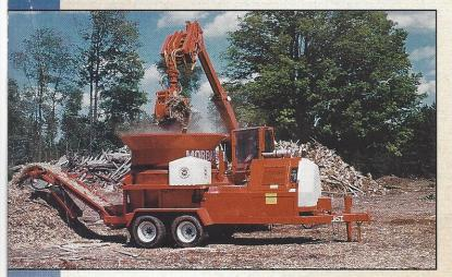
In designing the Model 950, Morbark engineers have filled an important niche in terms of both price and application. This unit is compact enough for easy transport and set-up yet heavy duty enough to handle a number of regrinding and primary grinding applications from bark, yard waste and brush to pallets and mill waste.
