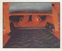
The Model 950 is offered with an optional fifth wheel towing arrangement and with a debris loading flange system to help prevent material from spilling during the loading process.
