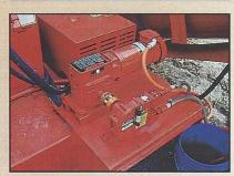
The fail-safe hydraulic system features a sensor which shuts off the feed of material in the event the auger is stopped for any reason.
