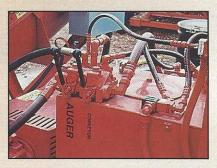
Water and colorant are mixed precisely in the control panel and injected into the mulch through six spray nozzles
