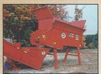
The rate of color applied per cubic yard of mulch is easily adjusted with the variable flow colorant metering pump. Changing colorant is simple too, just change drums and continue.
