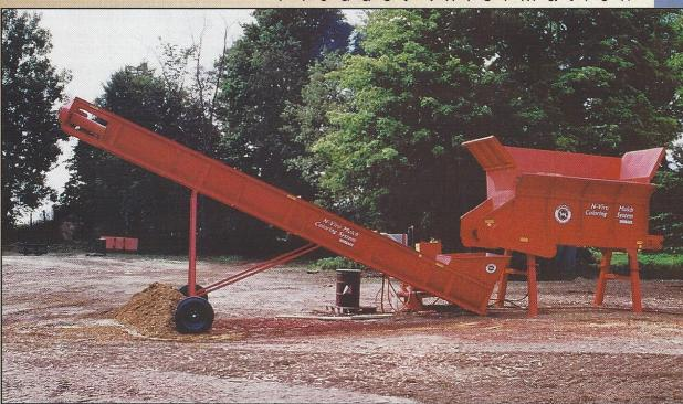
Now there's a better way to profit from shredded, recycled wood waste other than converting it into common boiler fuel, compost or animal bedding. The Morbark N-Viro Mulch Coloring System turns shredded wood waste into color enhanced, premium landscape mulch, a high value consumer product with a large profit potential. The Morbark N-Viro Mulch Coloring System employs a patented process
