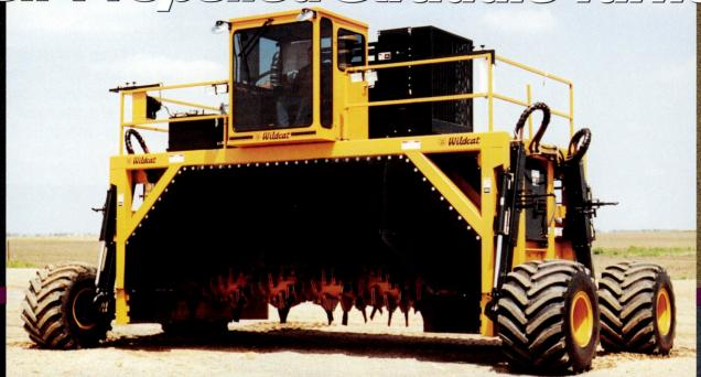
Wildcat Manufacturing Turner with optional four-wheel drive, forward speed control and reversible fan
