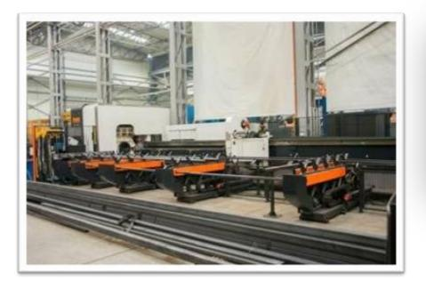
To make frames and many steel parts of all recycling machines, Pronar use 3D lasers which replace work of several others – drills, milling machines and saws. It is efficient, fast and cost saving.
