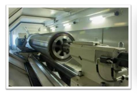
Pronar provides own shafts produced inhouse with solid shafts core which result in longer lifetime and ability to process harder material and stand higher pressure from hard materials.
