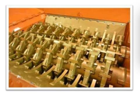
Pronar uses special type of Creusabro steel for shafts knives manufacturing. It has self hardening properties. The more impact from hard material on Creusabro steel, the harder it eventually gets.
