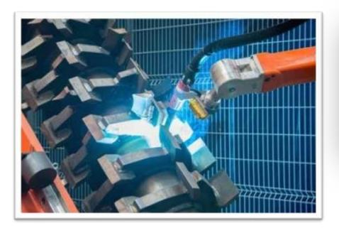
In Siemiatycze factory, where all recycling machines are built, automated welding robots are used. High repeatability and a perfectly routed weld are undoubted advantages.
