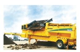
**GRIZZLY SCREEN OPTION.** The optional grizzly attachment can be mounted over the hopper to prescreen large materials and create more consistent overs material.
