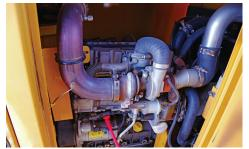
**EASE OF MAINTENANCE.** The TR5300 features a maintenance access platform for the Deutz TD 2.9L Tier 4 Final (Stage IV), 74 hp (55 kW) engine. With several access doors around the engine compartment, maintenance work on vital machine systems can be completed with minimal effort.
