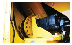
**DRUM DRIVE.** A hydraulic-driven chain drive system allows the drum to lift off the cog for service. Bolt-on sprockets can be changed quickly and help lower repair costs. Drum drive intelligently communicates with the infeed system to prevent overfeeding.
