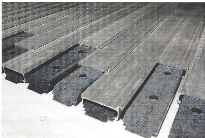
Live Floor unloads rapidly without bridging
